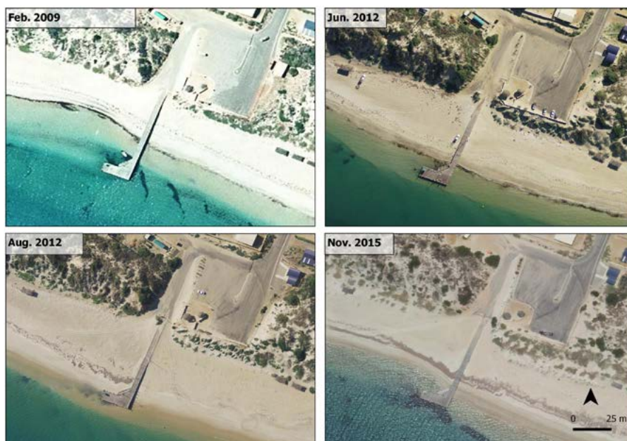
Figure 9.7: Variability in beach position and beach width at Port Gregory Jetty 2009-2015 (Source: Landgate)
