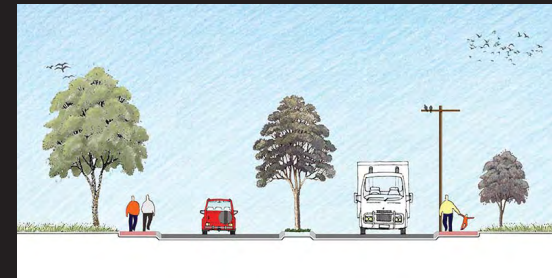
3 SECTION B: MAINSTREET TREE PLANTING IN ROAD VERGE & MEDIAN - TOWN APPROACH SCALE 1:100 @ A1
